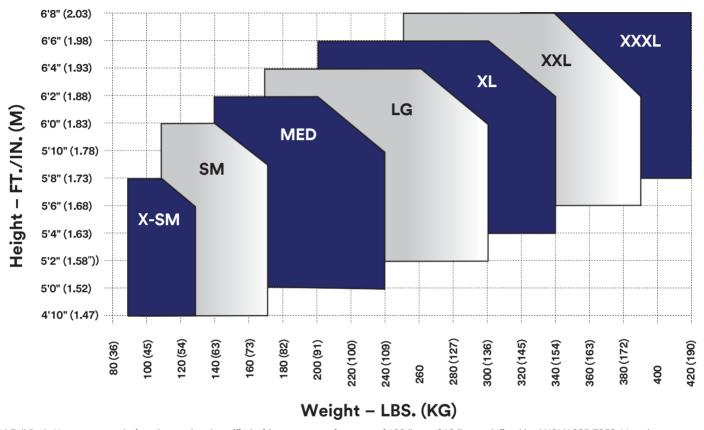
3M Full Body Harnesses are designed, tested and certified with a user capacity range of 130 lbs. to 310 lbs. as defined by ANSI/ASSP Z359.11 and up to 420 lbs. conforming with OSHA 29 CFR 1910.140 and 1926.502 regulations. For users below the weight capacity range of 130 lbs., the application shall be evaluated by the employer's Competent Person to determine alternate or applicable protection methods.
